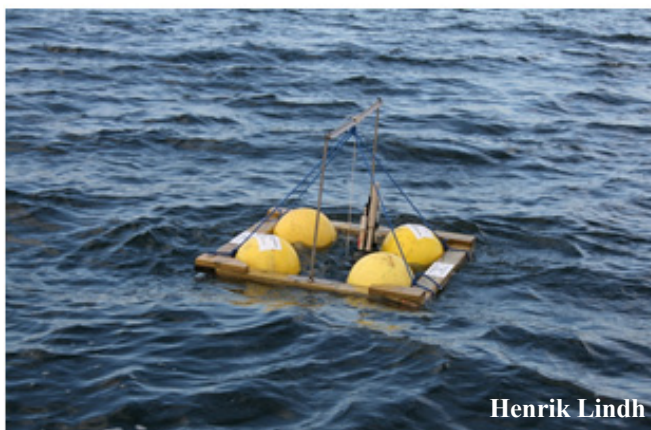
The top of the ARVOR-C, seen in the middle of the experimental float, has come up to the surface and transmits information to the satellite after a successful profile measurement
